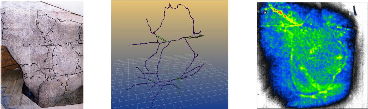
**Fig. 7:** Left: Manual mapped cracks on the cow of the Giebichensteinbrücke. Middle: 3D mapping of the cracks with the tracking system. Right: Phase image of a thermal sequence.
