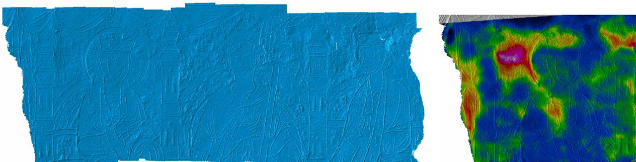
**Fig. 6:** Visualization of the plaster scratches. Left: triangle mesh as a result of photogrammetry. Right: overlay of a section with a thermogram that was recorded with higher resolution from the scaffold.
