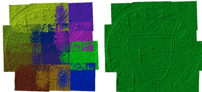
**Fig. 2:** Results of photogrammetric 3D capturing: Merging of single measurements (left) and the measurement result as 3D data set (right).
