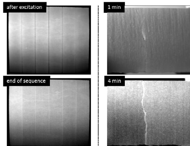
**Fig. 3:** Thermograms of Cottaer sandstone specimens with notches (left) and with a real crack (right) after 1 minute of heating with an IR radiator (top) and after 4 minutes of cooling down after heating (bottom). During cooling down, there is a contrast reversal: the notches and cracks appear warmer in relation to the environment.
