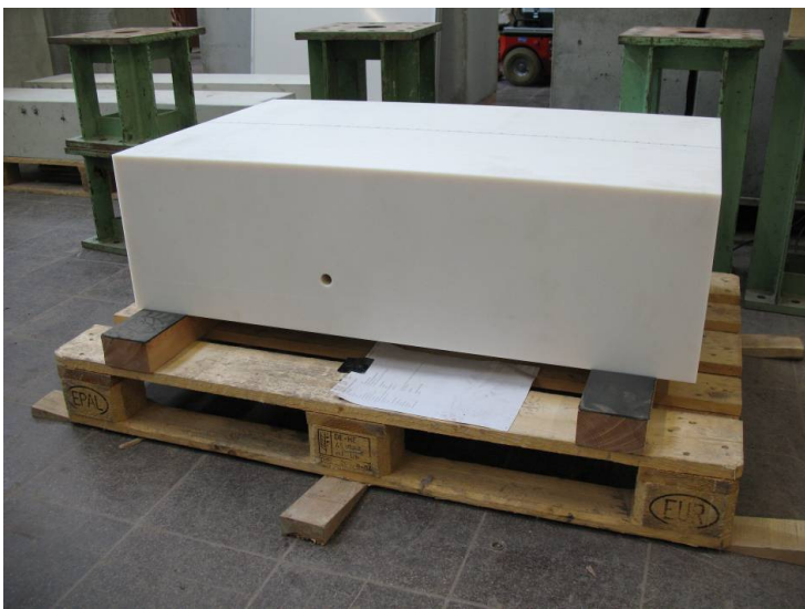
Fig 2 Reference specimen made of polyamide.
