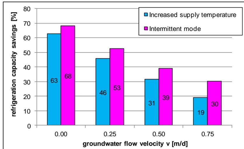
**Figure 3.5** Energy savings for different operating modes during the operating phase for the basic system depending on the groundwater flow velocity
