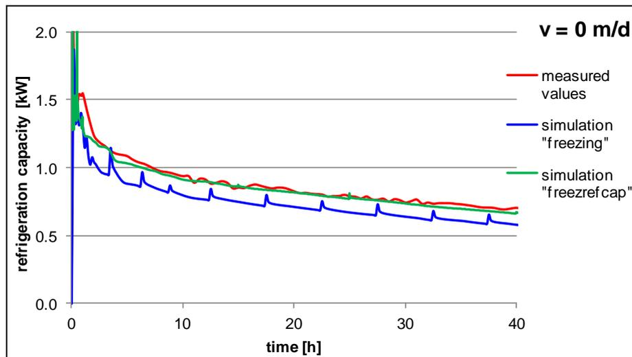
**Figure 3.3** Comparison of measured and simulated refrigeration capacity ( $v = 0$  m/d)
