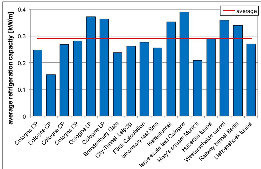
Figure 3.1 Comparison of average required refrigeration capacity in freezing phase
