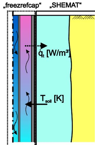
Figure 3.2 Interfaces between „freezrefcap“-module and SHEMAT
