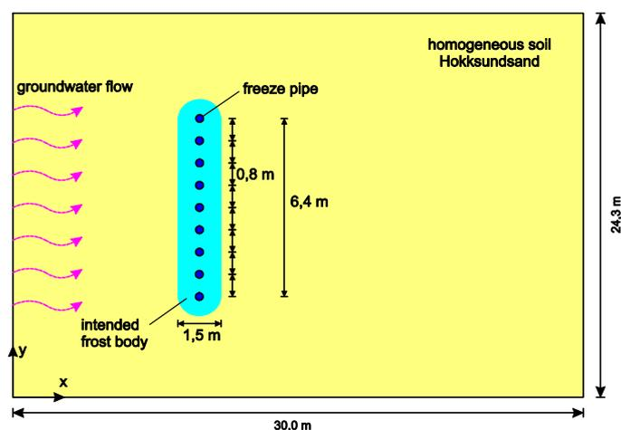
Figure 3.4 Basic system (excavation pit) for optimizing the refrigeration capacity
