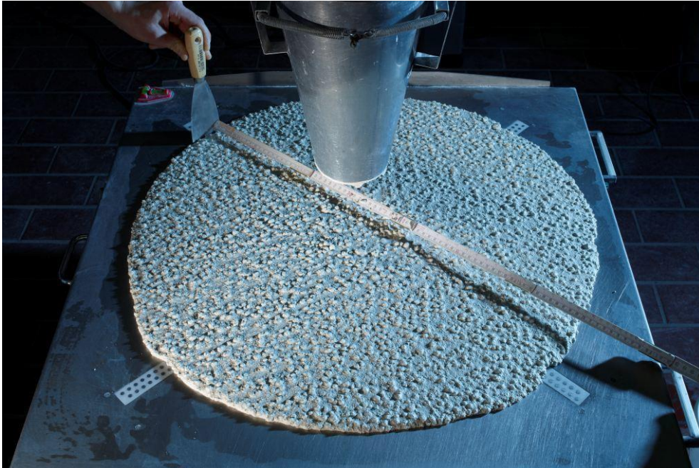
Figure 3: Slump flow of the optimised architectural lightweight concrete formulation
