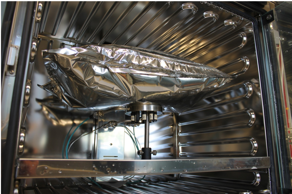
Figure 2: Testing sample with seal seam adapter in a climate chamber
