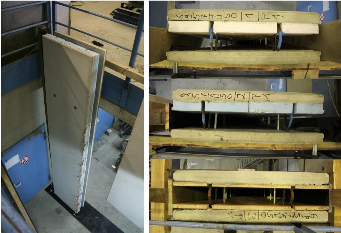
Figure 4: Vertical aligned sandwich wall and top view of test bodies.jpg
