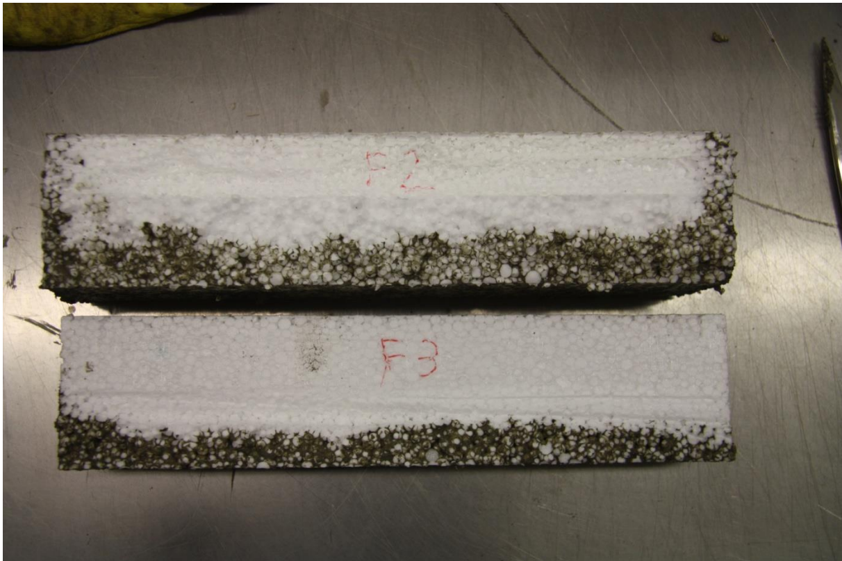
Figure 1: Dark coloring of EPS due to absorbcency of the water-cement mixture.jpg
