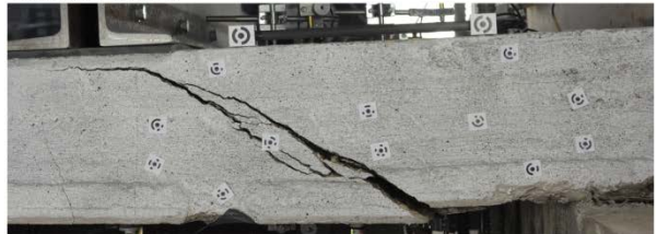
Figure 6: bruch.png Figure text: Results of the photogrammetric evaluation of the crack development during the in-situ loading test
