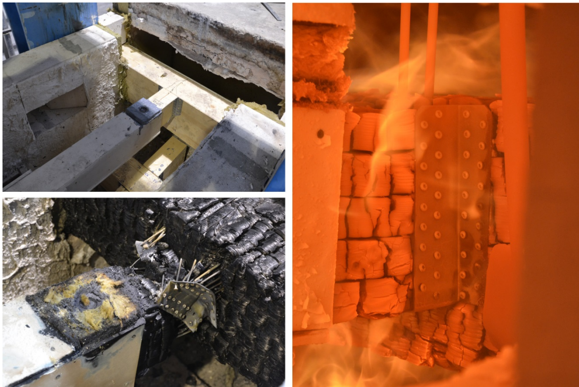
Figure 6: fire tests with joist hangers: left side: one specimen before and after the test, right side: Looking into the furnace during the test
