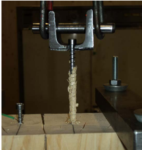
Figure 3: Investigation of the pull out resistance of full thread screws in regard to the temperature
