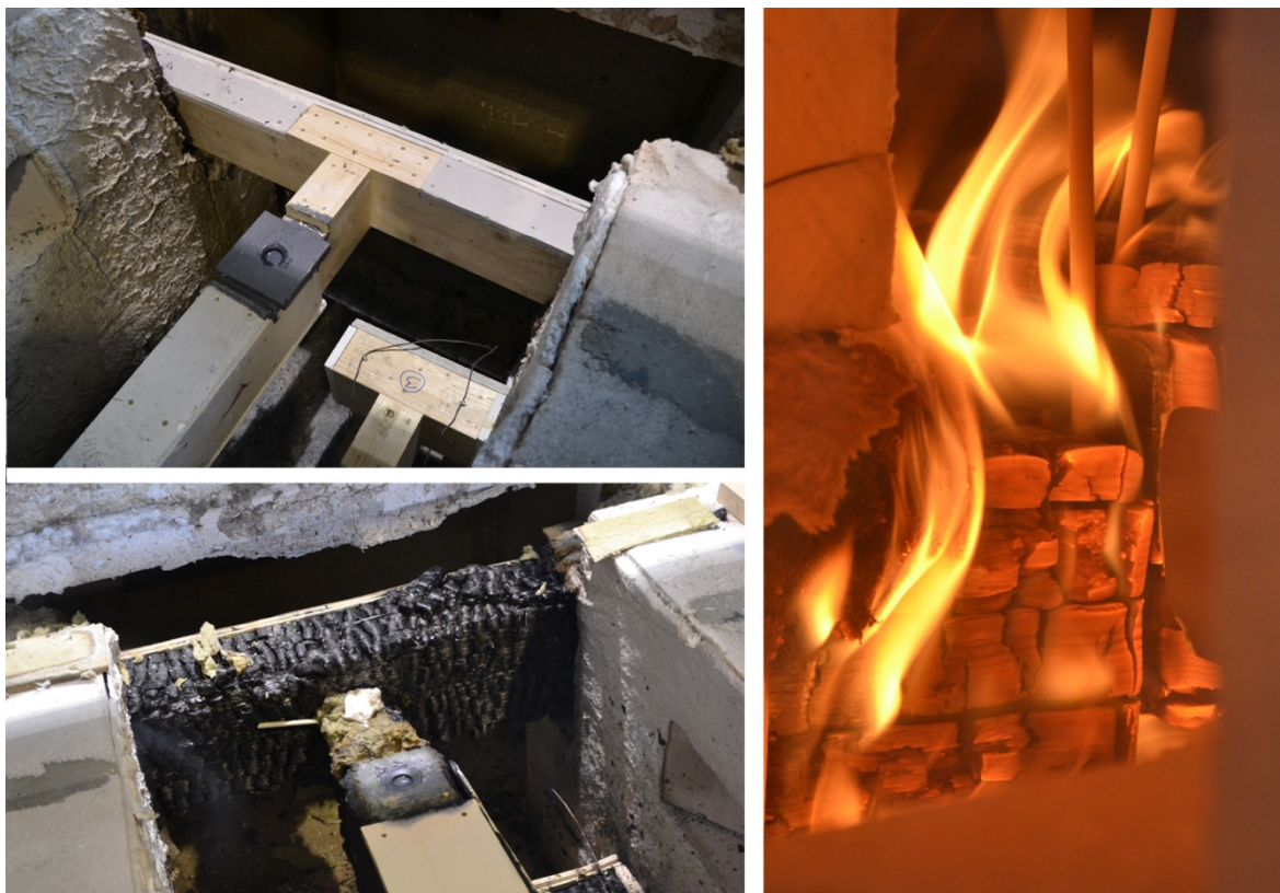
Figure 7: fire tests with pairwise crossed full thread screws: left side: one specimen before and after the test, right side: Looking into the furnace during the test.
