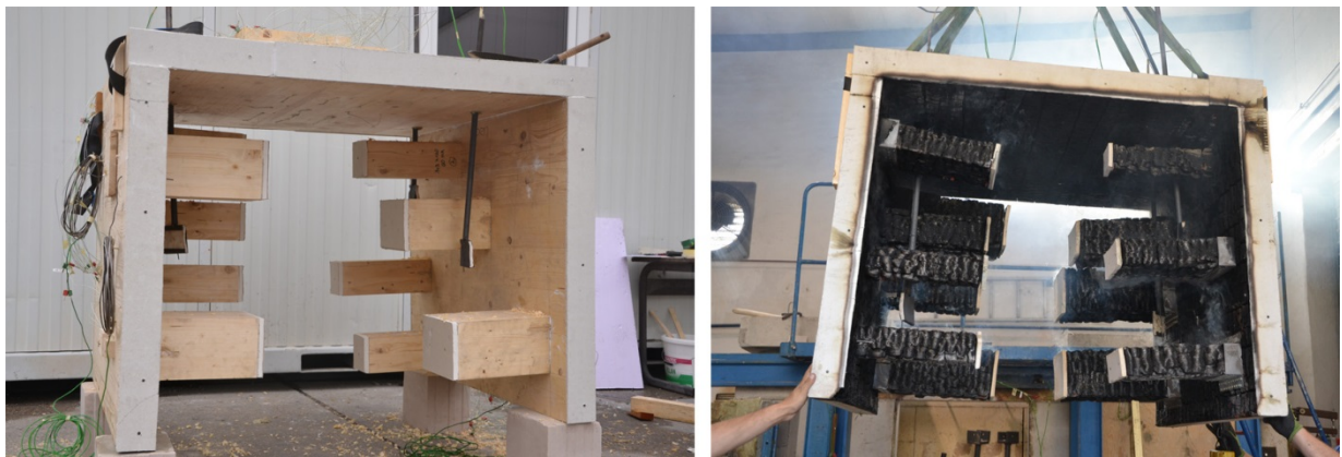
Figure 2: Specimen for the unloaded fire tests. Left: before the test, Right: After the test.
