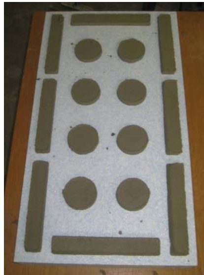
Fig. 2: Insulation board coated with adhesive mortar prior to attachment to the base wall (portion of the coated area 40 %). In order to reach exactly equal conditions for all measurements, the mortar was applied using a stencil.
