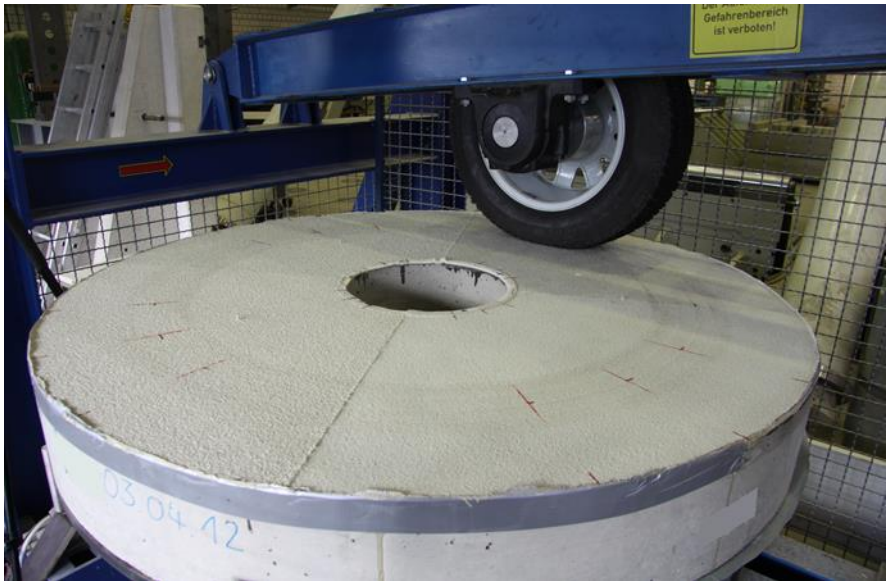
Image 3: Test bench Driving Abrasion Test (DAT)
