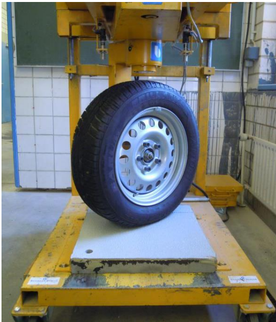
Image 2: Test bench Parking Abrasion Test (PAT)
