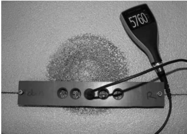
Image 5: Magnetic inductive method – device for coating thickness measurements
