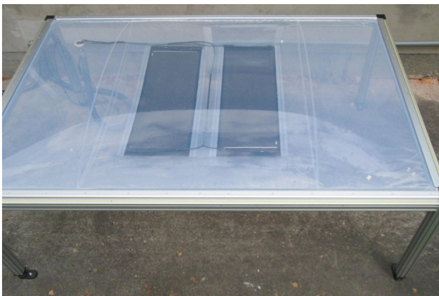
Fig. 2: Outdoor exposure stand of the ETFE cushions prototype with interior PV modules
