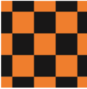
Fig. 3: Resonator arrangement "8|8" on 1.5 mm thick steel plate with 25 cm edge length (orange: resonators; black: bare plate). © Fraunhofer IBP
