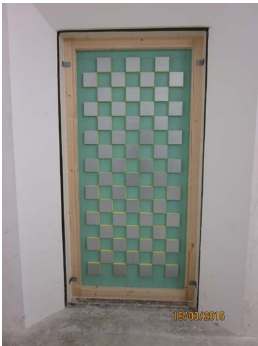
Fig. 5: Plasterboard with 56 resonators (1.5 mm steel on 25 mm Sylomer, edge length 10 cm) in the opening of the door testing facility. © Fraunhofer IBP
