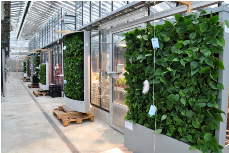
Pic. 2: Experimental setup in the greenhouse - six different indoor greening systems with planting on scales
