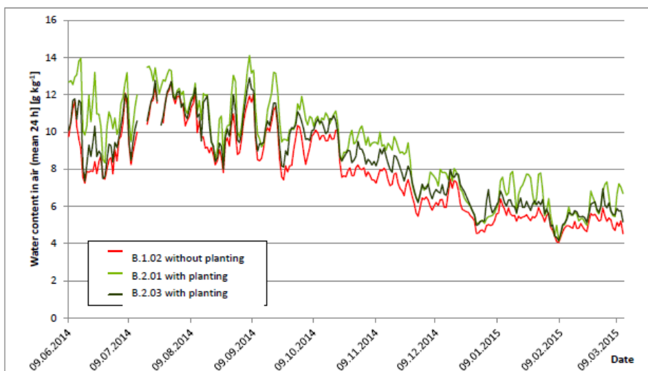
Pic. 6: Comparison of water content in air (mean 24 h) in small offices with greening (B.2.01 with closed door and B.2.03 with open door) and without greening (B.1.02 with open door) in the period of 09.06.2014 to 12.03.2015
