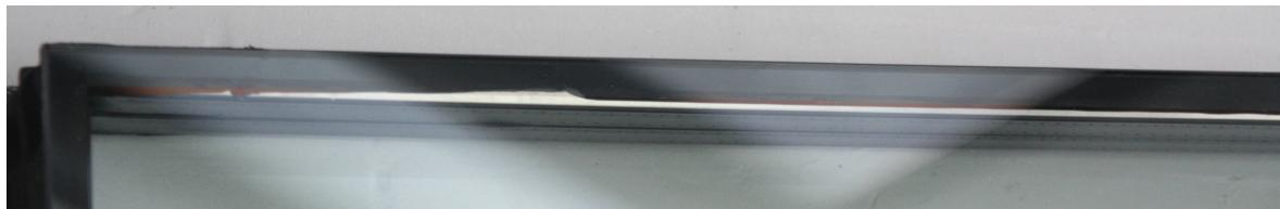
**Figure 4** Insufficient butyl covering on a spacer
