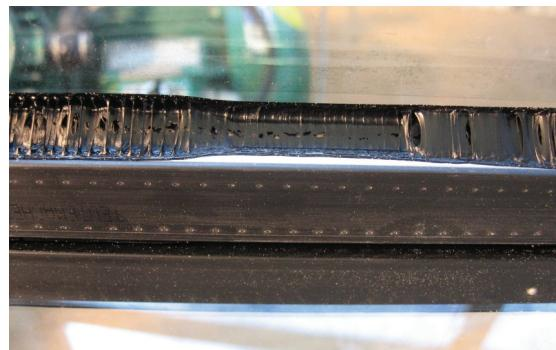
**Figure 7** Example of stringing in butterfly test: patches with bad adhesion between butyl and spacer are visible
