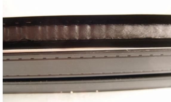
**Figure 8** Cohesive failure in the butyl – no stringing
