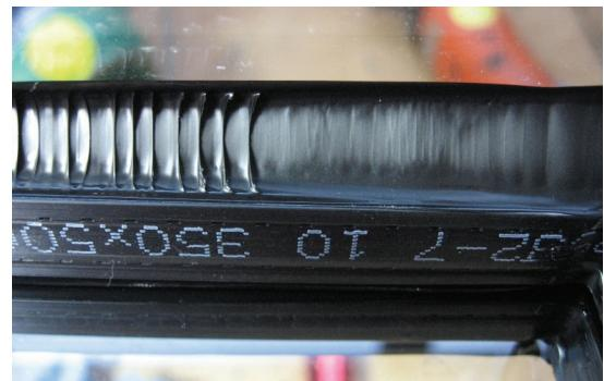
**Figure 6** Example of butyl stringing in butterfly test: good adhesion – formation of a closed curtain of strings
