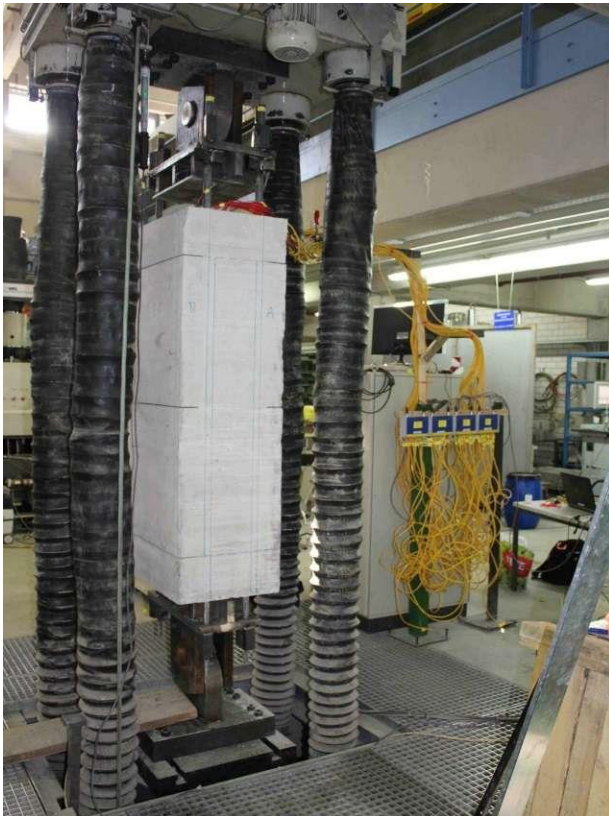
Figure 5: Experimental setup for tension member tests
