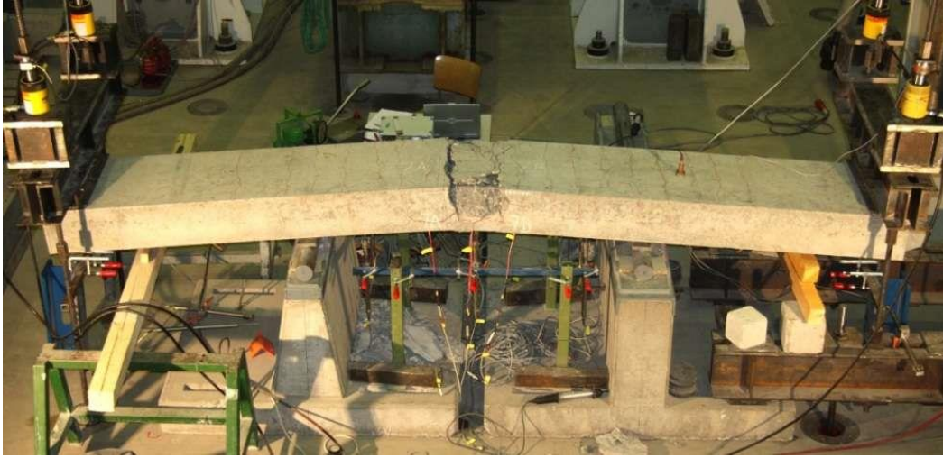
Figure 2: Experimental setup for reference and trial tests with test bodies after trying
