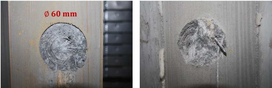
Figure 3: Shearing of the HPC dowel, shown in each composite part
