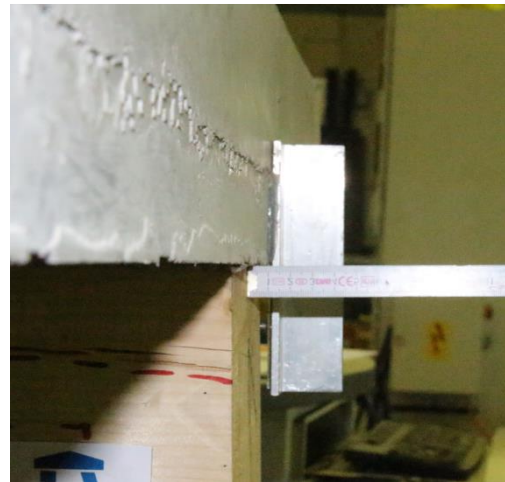
Figure 7: Slip between the two composite parts at the beam end showed in simulation (left) and in test (right)
