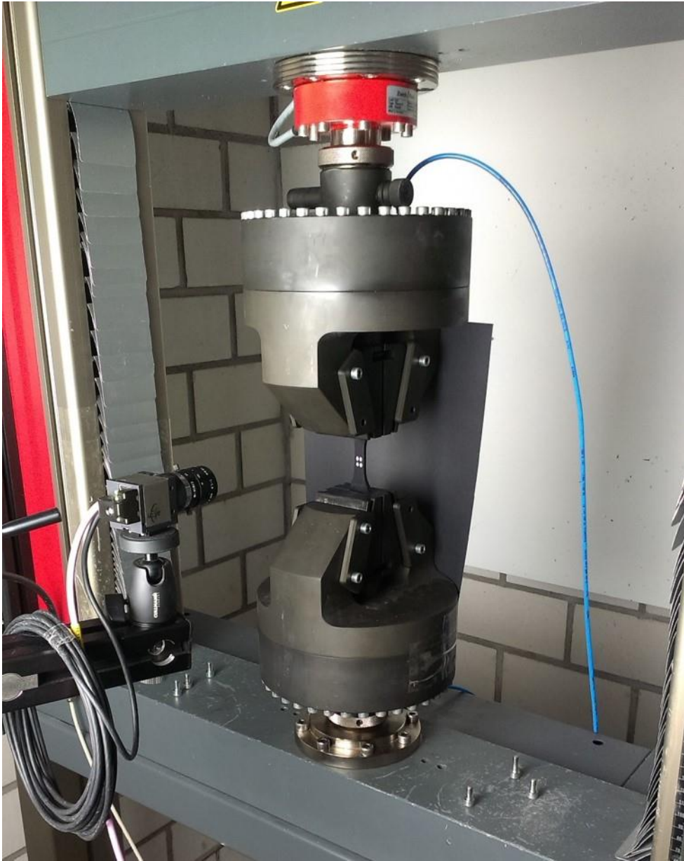
Bild 5: uniaxiale Zugprobe.jpg Experimental setup of tension test with optical measurement system
