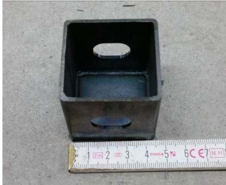
fig.4: RZ_Bild 4.jpg Turnbuckle of the connecting system 2
