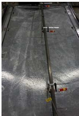
fig.5: RZ_Bild 5.jpg Wall element in negative pressure test shortly before reaching load capacity
