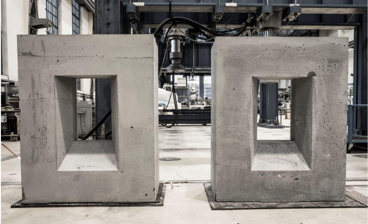
Figure 4: prototype 2, window element, ILC with a dry density of 800\text{kg/m}^3 (left) and 600\text{kg/m}^3 (right)
