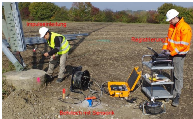
Figure 4: Parallel Seismic measurements to determine the length of foundation piles at an electricity tower. File: Figure4.jpg
