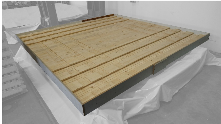
Figure 2: CLT-element with notches as shear connectors
