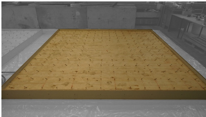
Figure 3: CLT-element with inclined screws as shear connectors. The screws are aligned along the expected principal shear forces.
