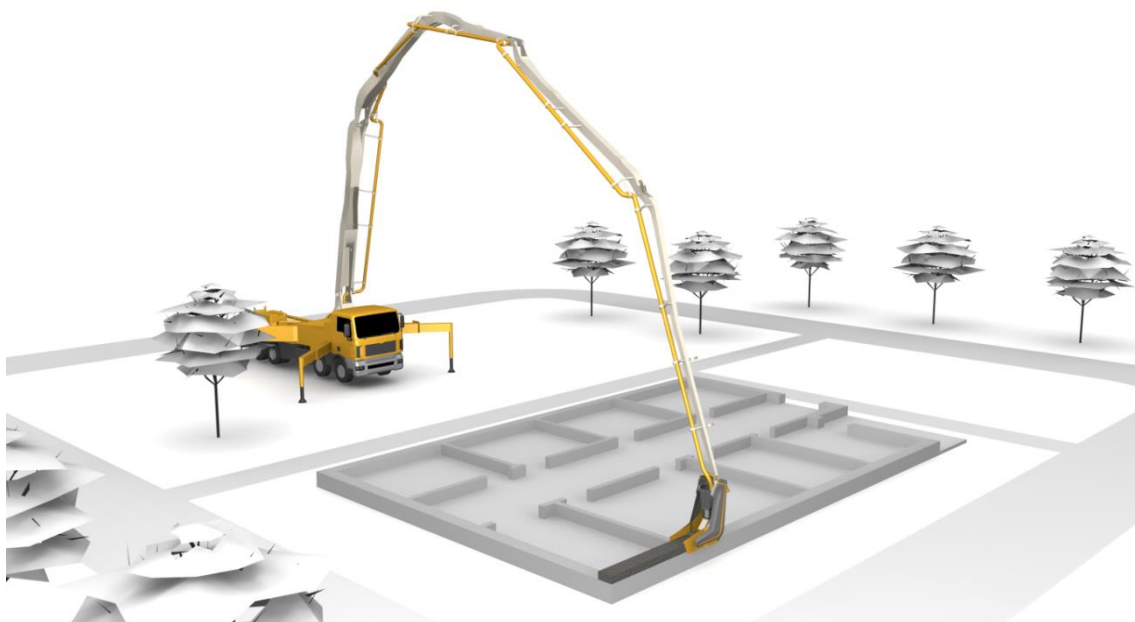
Figure 2: Concrete 3D printing directly on the construction site (animation)
