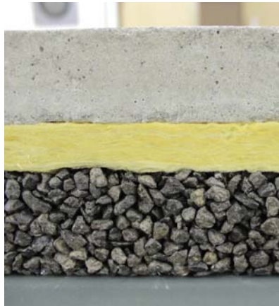
Fig. 3: Example of one of the investigated fills (side view of the ceiling covering). From top to bottom: cement screed (thickness: 43 mm), impact sound insulation slab made of mineral wool (thickness: 25 mm), basalt grit fill with a grain size of 5 – 8 mm (thickness: 60 mm).
