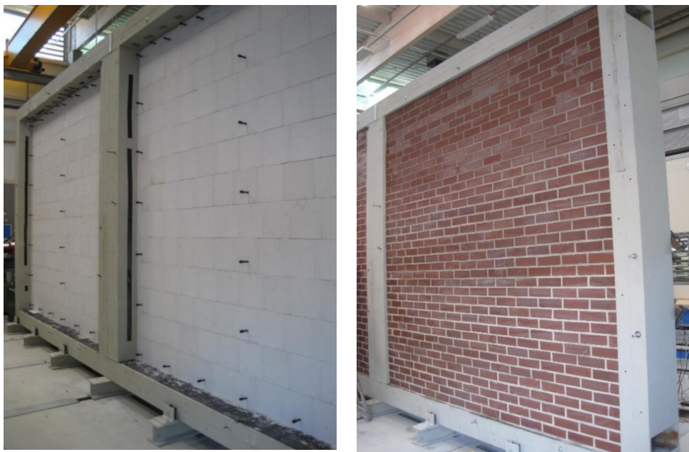
Figure 6 Testing the line anchoring system (left position of the vertical anchor lines; right the finished test arrangement)
