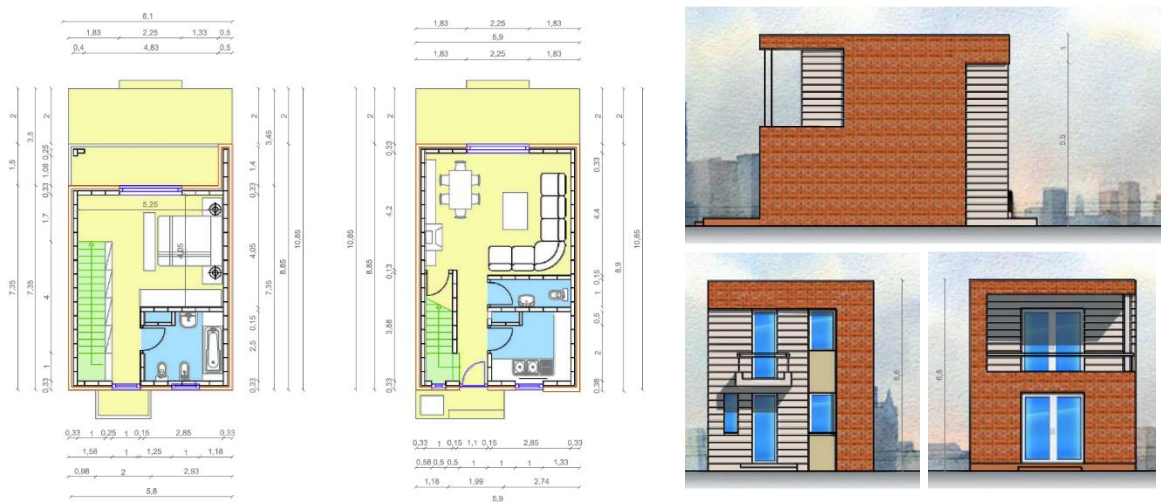
Figure 5 Design of the Muster house: Two levels, entrance, living room, kitchen, WC, stairs, bedroom, Bathroom, dressing room, balcony and terrace, Constructed area= 52,51 \text{ m}^2 = 8.9 \text{ m} \times 5.9 \text{ m} , height 6.8 m
