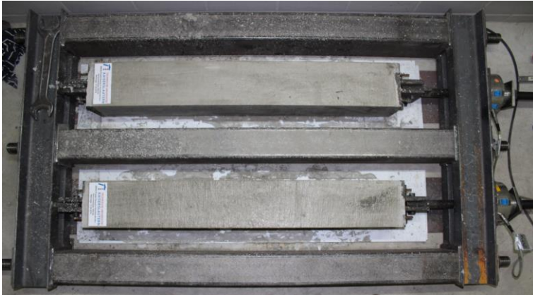
Figure 2: Dauerstandversuch.bmp Setup for the measurement of the restraint forces
