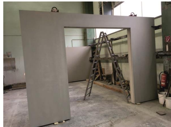
Fig. 6: sandwich panel with gate opening
