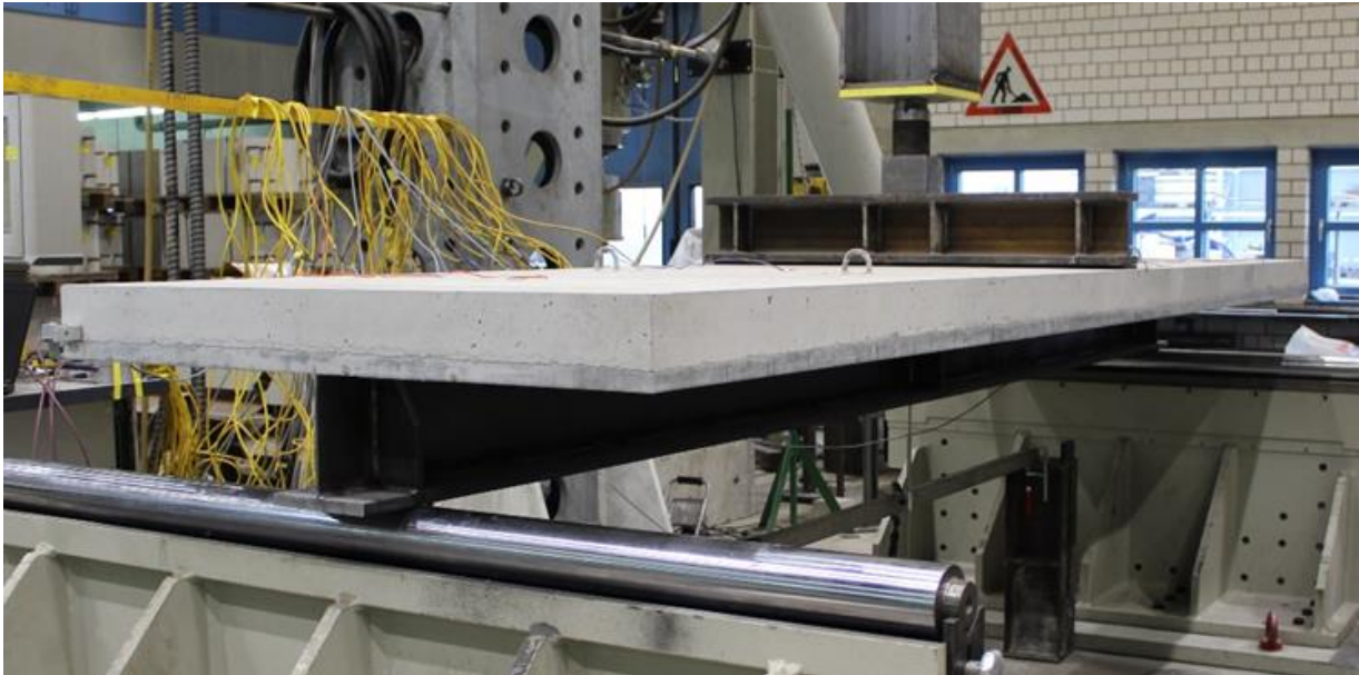
Figure 6: Test setup, 3-point bend experiment
