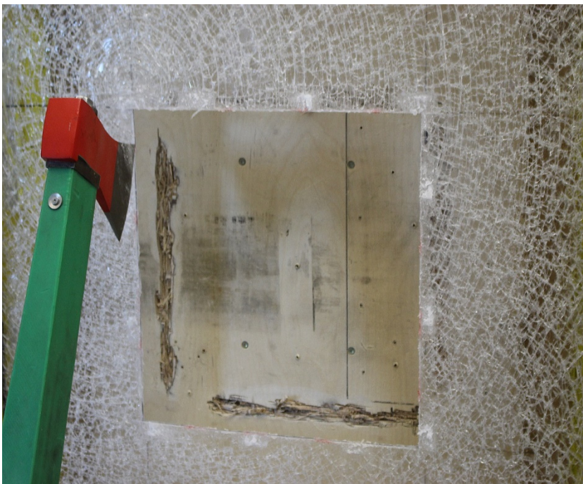
Figure 3 Test with the axe on a thin glass-polycarbonate composite panel with thin glass Optiwhite.
