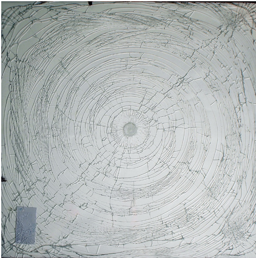
Figure 2 Fracture pattern of the attack side of a thin glass-polycarbonate-composite panel after the impact of the steel ball.
