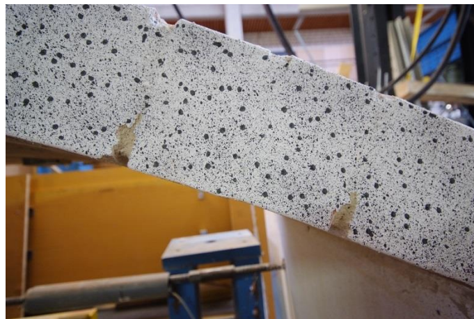
Failure pattern of the vault at the one-third-way position
