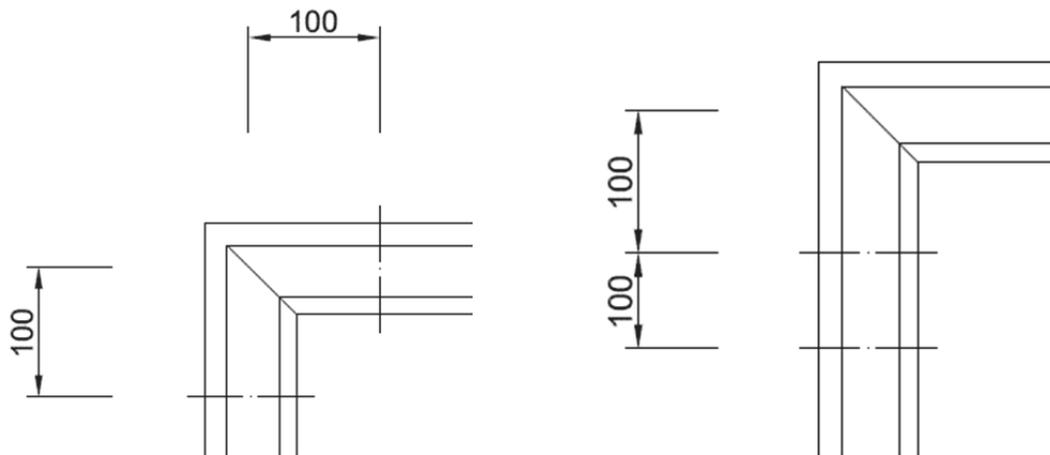
**Figure 8** Group fastening for better load transfer with "point loads"
