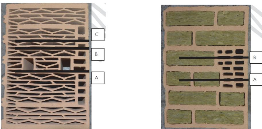
**Figure 6** Reveal brick with pattern of cavities optimised with respect to the mechanical properties.
