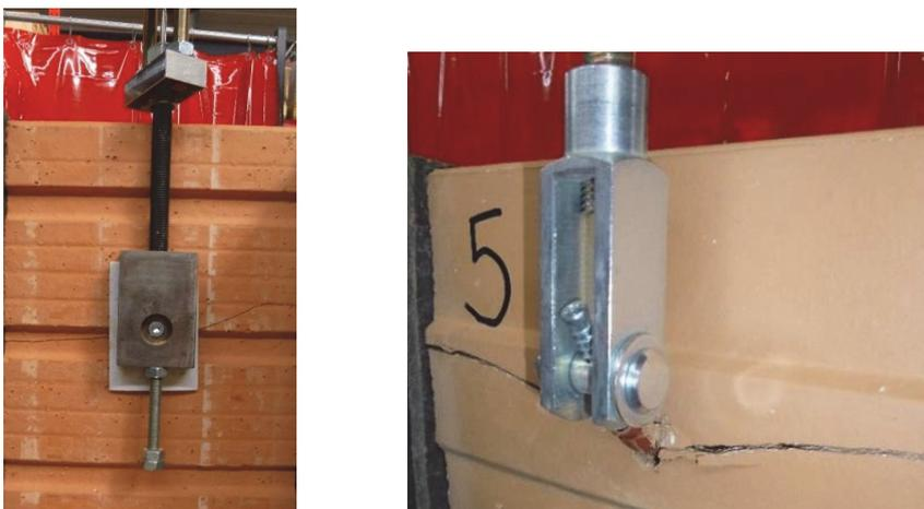
**Figure 2** Test for determining the load-bearing capacity of the fastening
