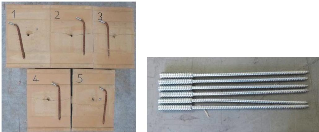
**Figure 11** Appearance of the fixing material at the end of the respective test
