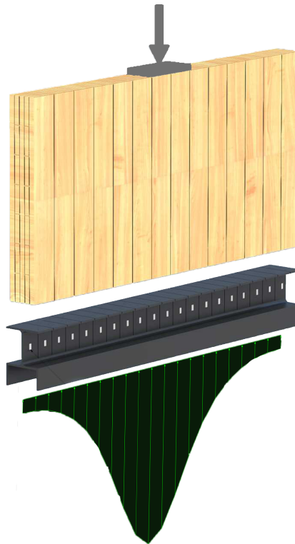
Abbildung 2.2: Load distribution by a single load in-plane
