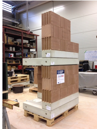
Figure 3 Assembling and locking the individual elements for model bodyshell construction
