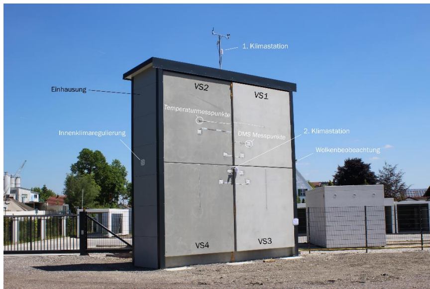
Figure 2: Test setup with facing shells VS1-VS4 (south-west orientation)
