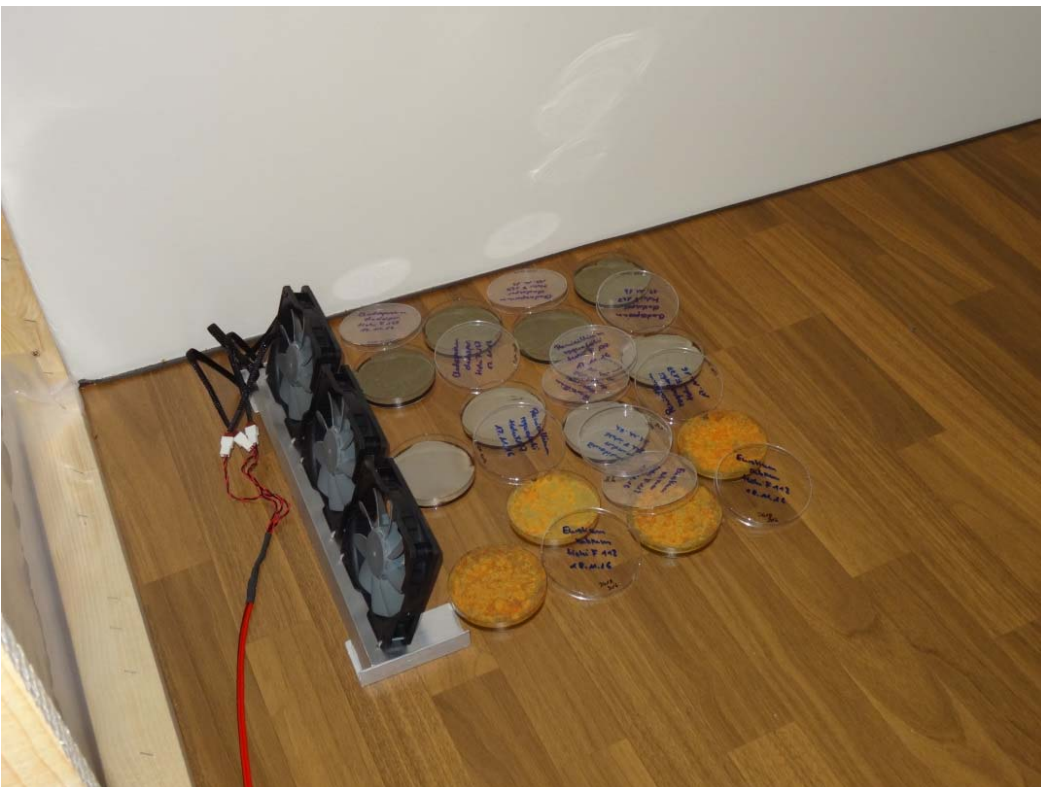
Figure 4: Ventilation system together with sporulating fungal cultures in a test room.
