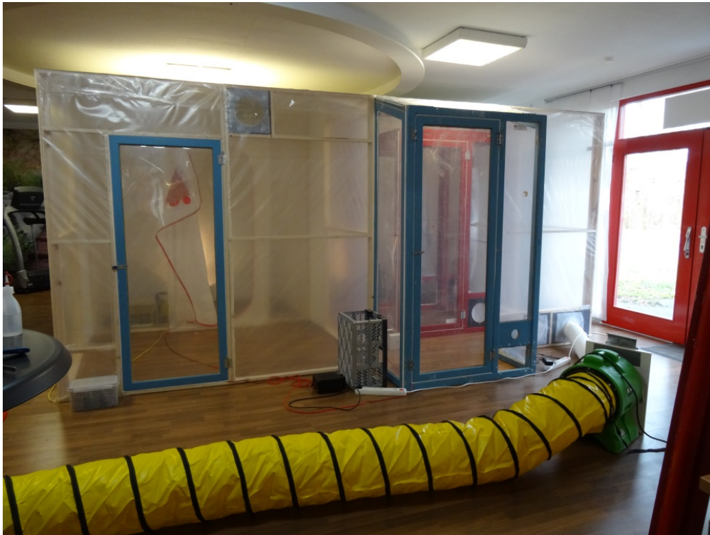
Figure 1: Total experimental setup with view at the anterooms; behind the test rooms with different partitions / double doors can be recognized on the right hand side.
