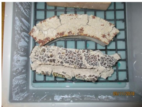
Figure 1. left unsuitable injection material in the over water storage (Roman cement), right needle-shaped crystals grow throughout the structure
