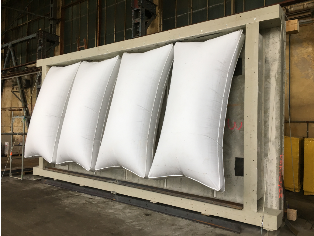
Fig. 5 Test framework of airbag test without test wall (the airbags become completely inflated between the interspace in the installed state)
