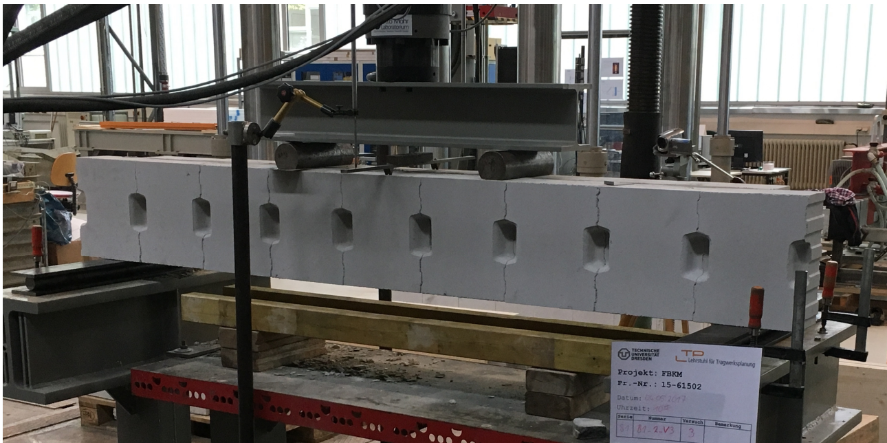
Fig. 1 CFRP textile reinforced bending beam made of calcium silicate masonry units Figure by Maik Erler, Bild01.jpg
