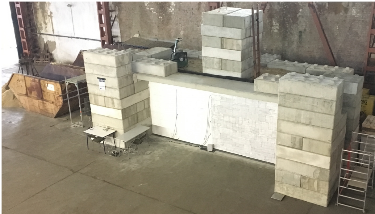
Fig. 4 Large-scale test setup of textile reinforced basement masonry under earth pressure after the performance of the test Figure by Maik Erler, Bild04.jpg
