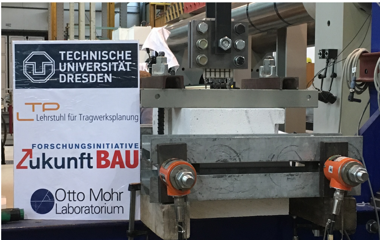
Fig. 2 Textile pull out test of CFRP textile out of autoclaved aerated concrete bed joint with imposed load Figure by Maik Erler, Bild02.jpg
