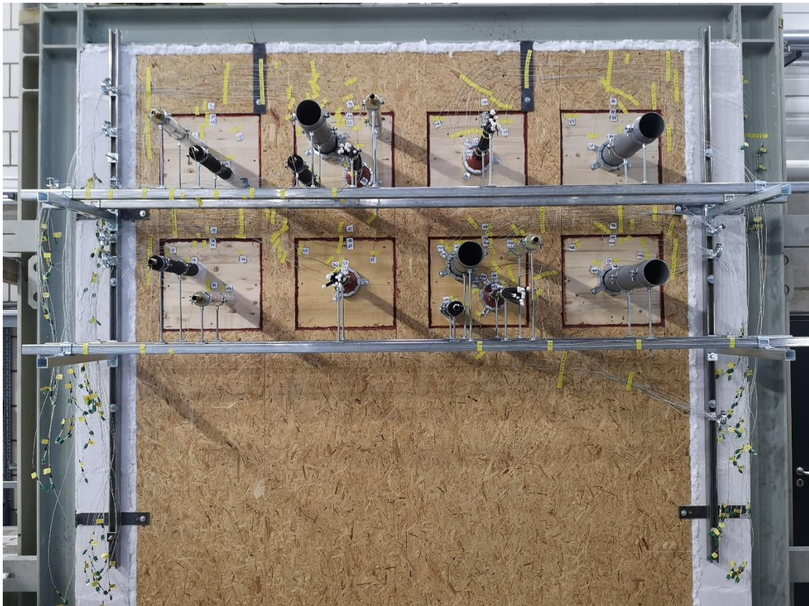
Fig 1: Full scale fire test, frame wall with penetration sealing systems
