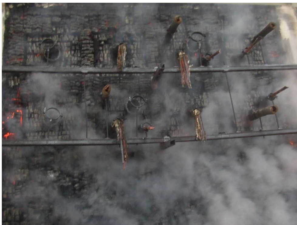
Bild 5: Full scale fire test, CLT wall while extinguishing
