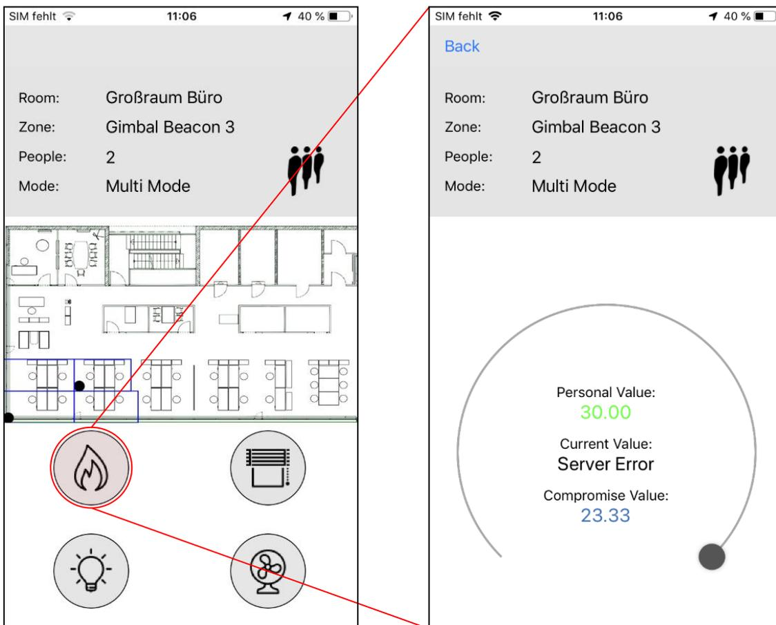
**Figure 2.3** Prototypical user interface of the application with main page and exemplary detail view (Left: Main-ViewController [Source (original map): Robert Bosch GmbH], Right: Sensor-ViewController)
