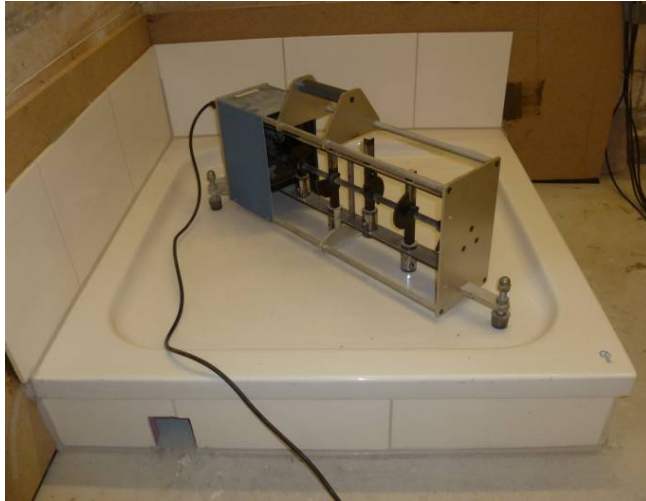
Fig. 3: Excitation of a completely mounted and tiled shower tray, using a tapping machine.
