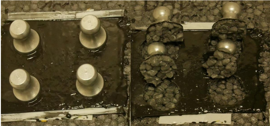
Figure 2: Front pull-off test before and after measurement, modified ETICS adhesive on EPS at 2 mm test layer thickness
