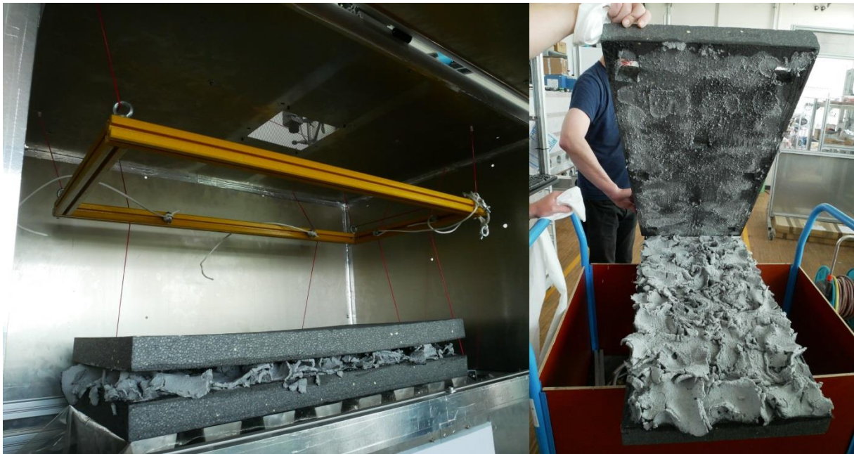
Fig. 5: Decapped EPS plate after microwave irradiation in MAC-RTM at a surface temperature of the adhesive of 80 °C
