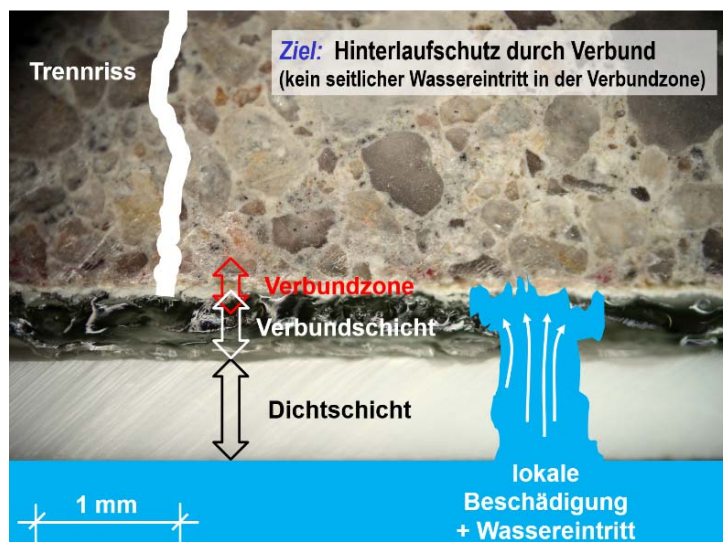
Figure 2: A schematic representation of the functional principle of a FBV system [source: DBV-Heft 44]
