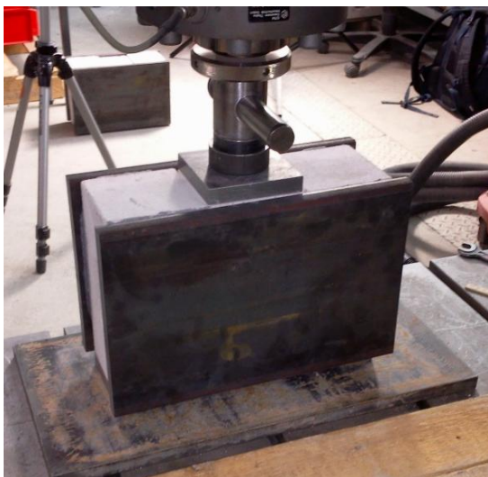
Figure 7 Modified test procedure B with bonded steel plates before load Initiation left and after failure right
