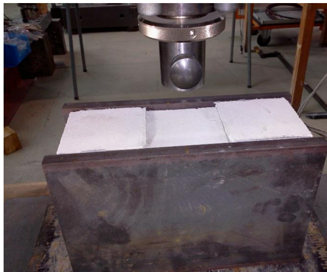
Figure 7 Modified test procedure B with bonded steel plates before load Initiation left and after failure right
