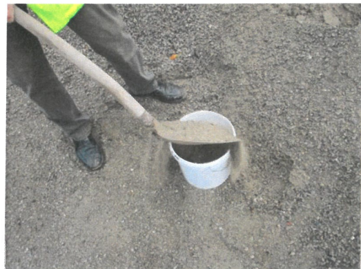
Figure 7 Sampling of aggregate material 0/16 concrete chips on the site of the company Heim Deponie & Recycling GmbH
