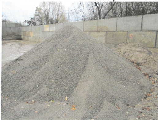
Figure 7 Sampling of aggregate material 0/16 concrete chips on the site of the company Heim Deponie & Recycling GmbH
