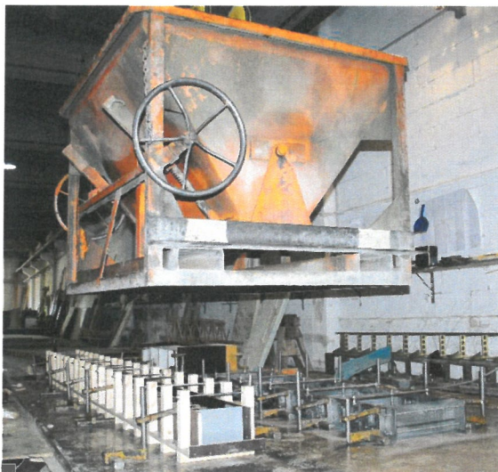
Figure 10 RC beams, concreting process
