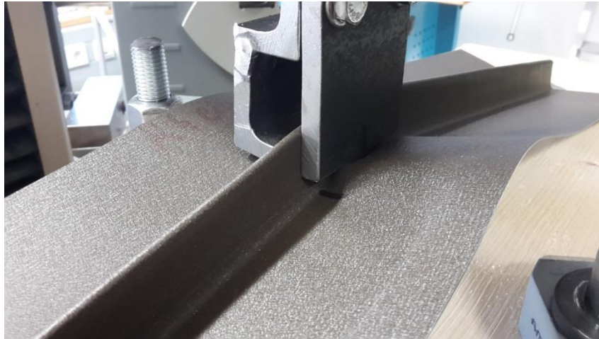
Fig. 5: fig 5 – failure pattern wind suction test.jpg Investigation of the most unfavorable load situation with maxi-mal clamp distance. Failure pattern.
