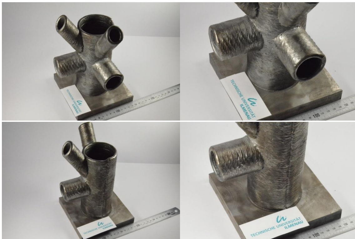
picture 1: Additively produced top flange knot with vertical and diagonal bars
