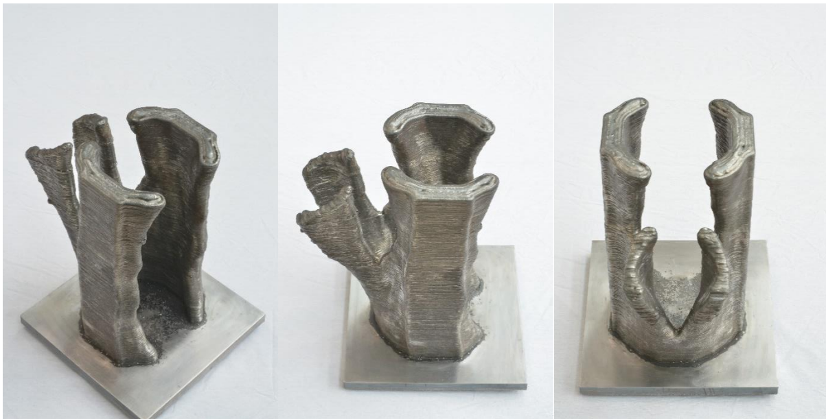
picture 4: additively manucured, topologyoptimized 30° diagonal joint
