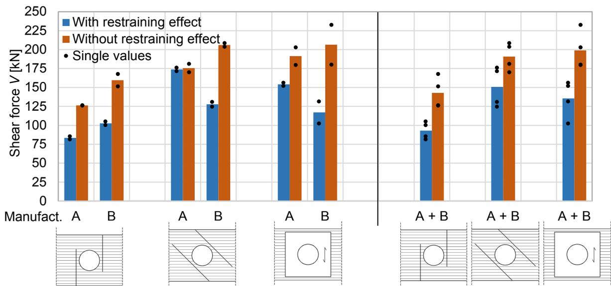
Figure 5: Failure loads of member group "Holes" ( $b \times h = 140 \times 700 \text{ mm}$ ,  $h_d/h = 0.4$ )
