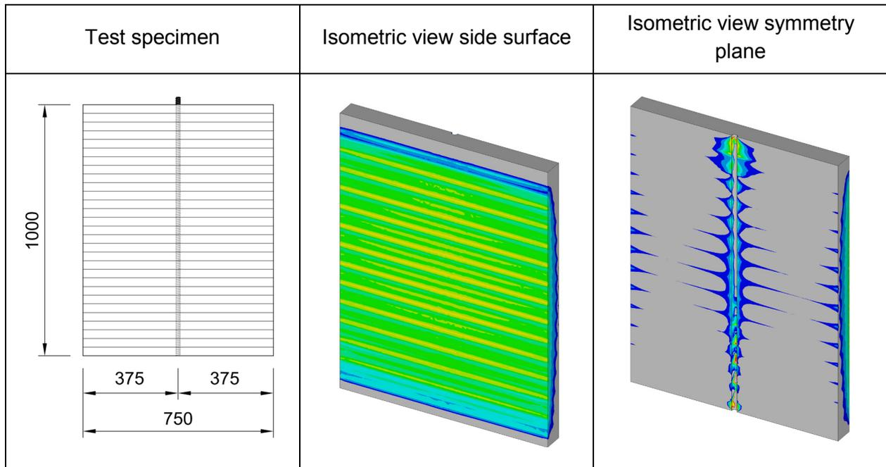
Figure 6: Stressed volume in tension perpendicular to the grain of an exemplary test specimen
