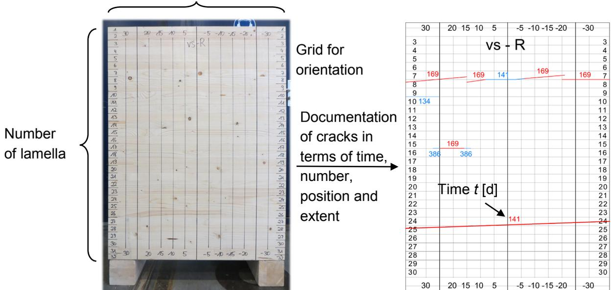
Figure 2: Exemplary documentation of crack occurrence on the rear side of a specimen
