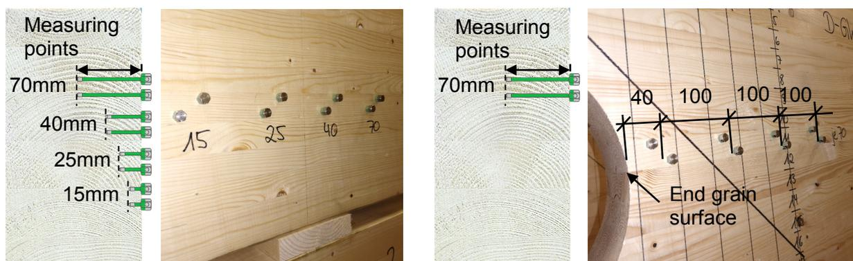
Figure 1: Situations of measuring the distribution of wood moisture by resistance measurements
