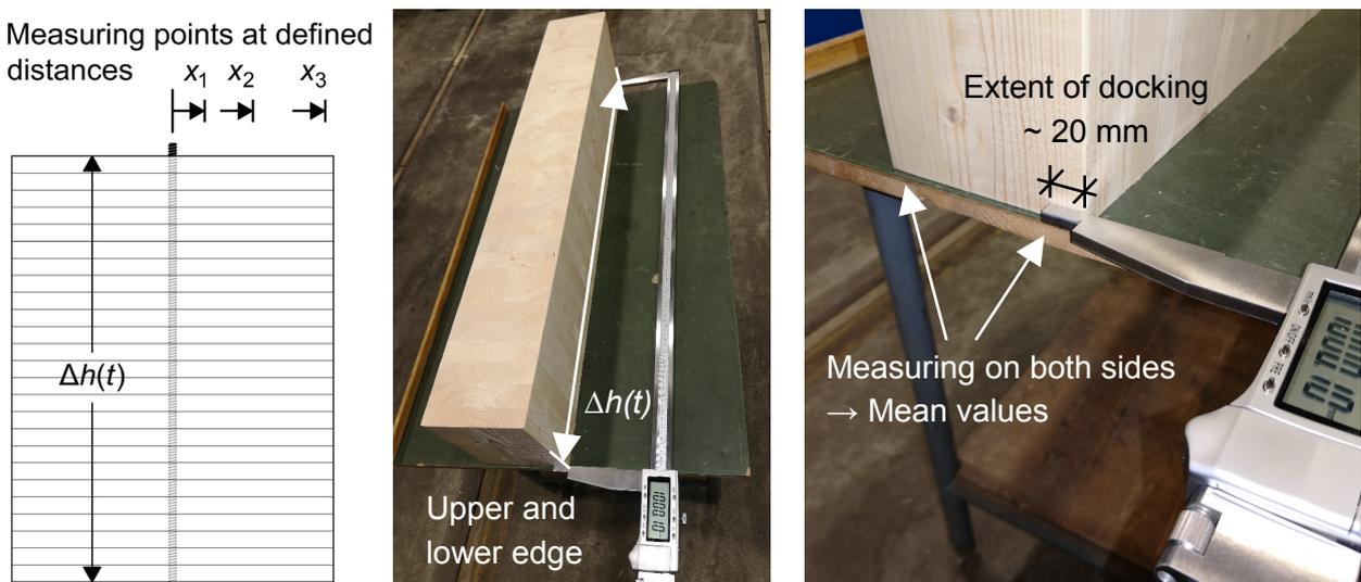
Figure 3: Measuring shrinkage deformations between upper and lower edge of the test specimen
