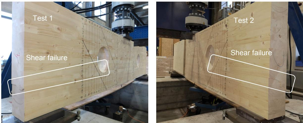
Figure 4: Exemplary shear failure of a beam with holes
