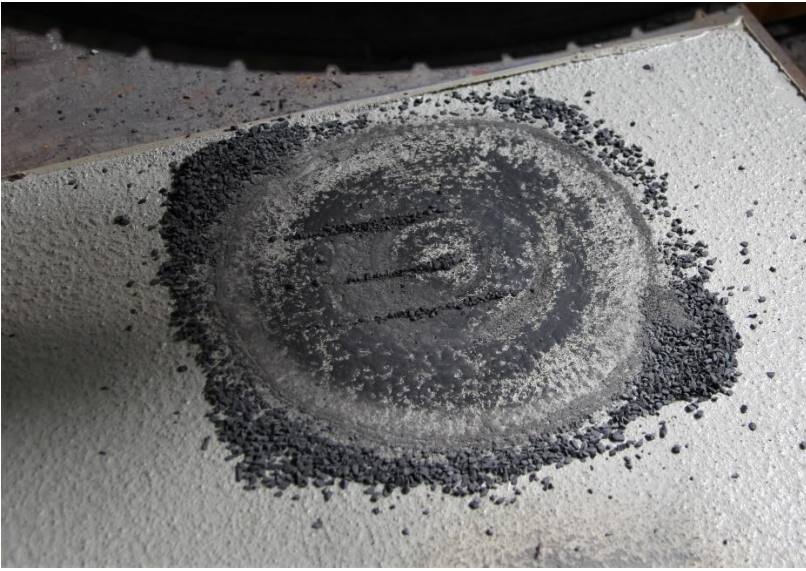
Figure 3: Implementation of the Parking Abrasion Test under the influence of grit
