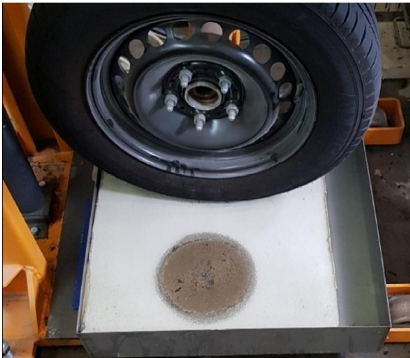
Figure 2: Parking Abrasion Test under water saturation
