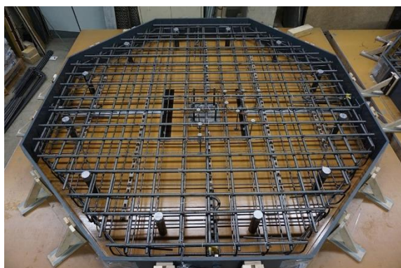
Figure 1: Reinforcement with formwork (left) and used steel fibres (right)
