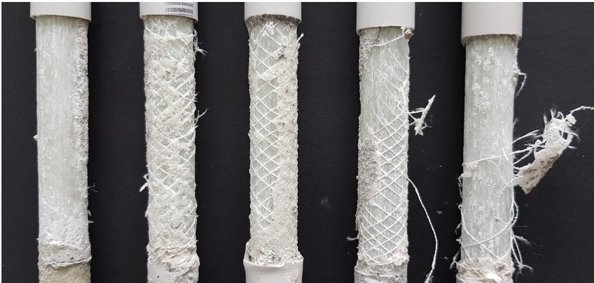
Figure 4: Time-dependent decomposition of the surface profile of GRP2 at 60°C. From left to right decreasing load with increasing service life.
