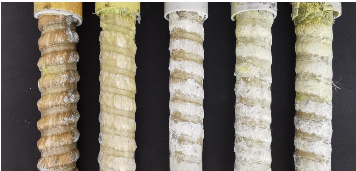
Figure 5: Time-dependent decomposition of the surface profile of GRK3 at 60°C. From left to right decreasing load with increasing service life.
