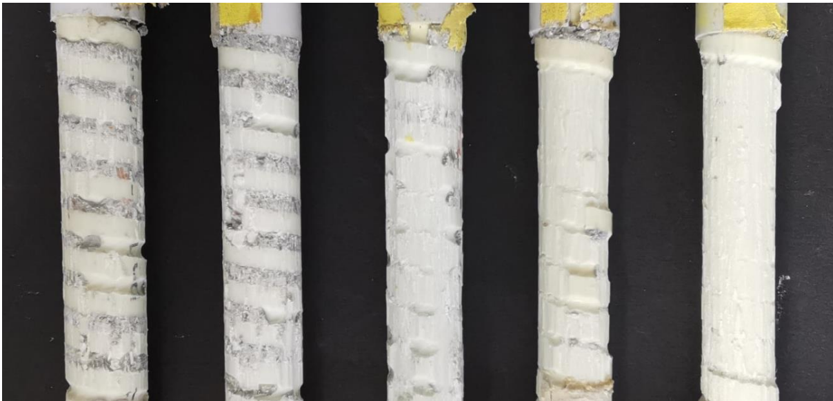
Figure 3: Time-dependent decomposition of the surface profile of GRP1 at 60°C. From left to right decreasing load with increasing service life.
