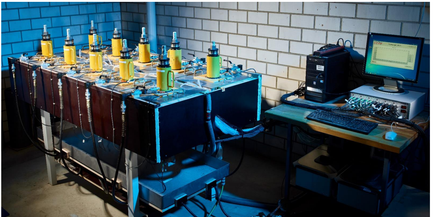
Figure 2: Test bench developed to analyse the time-dependent bond strength under continuous load and the external influences of moisture, increased temperature and concrete alkalinity.
