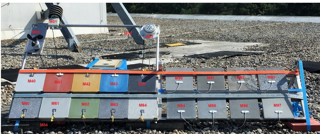
Figure 3: Test rig for determining the surface temperature of UHPC façade panels
