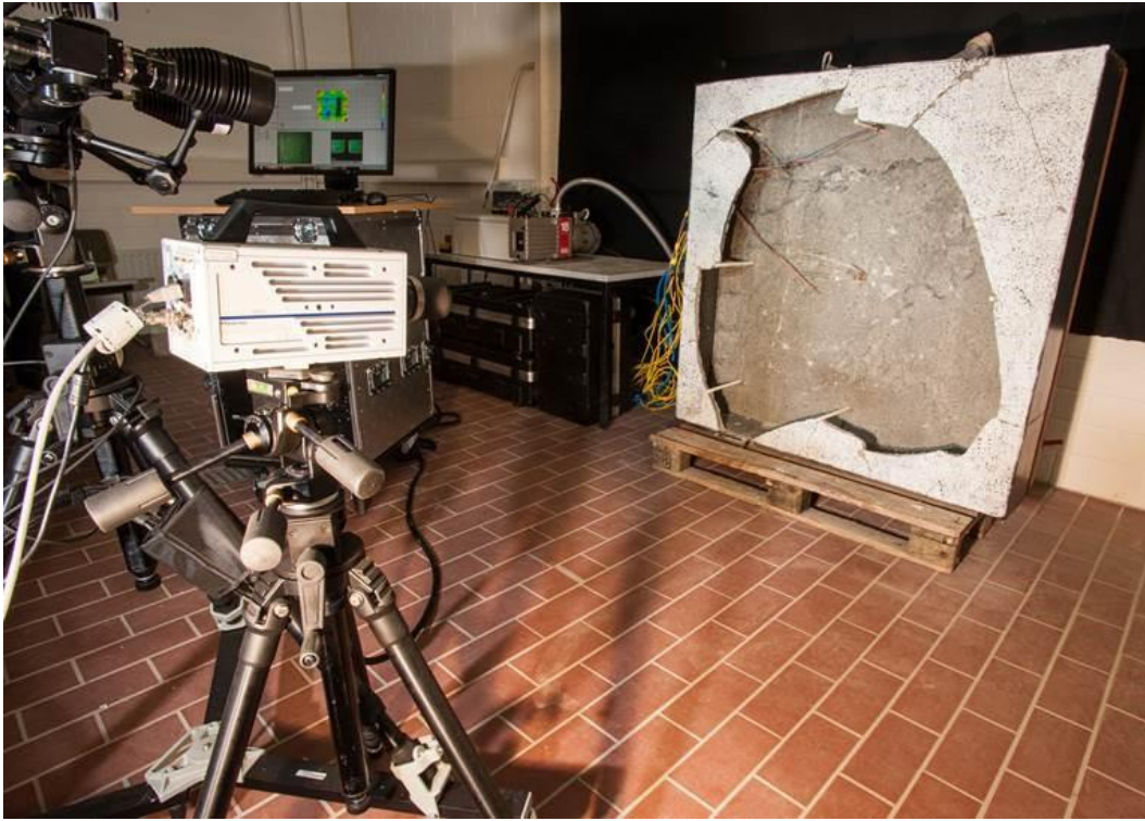
Figure 4: Test set-up for negative pressure tests on façade panels made of ultra-high performance concrete
